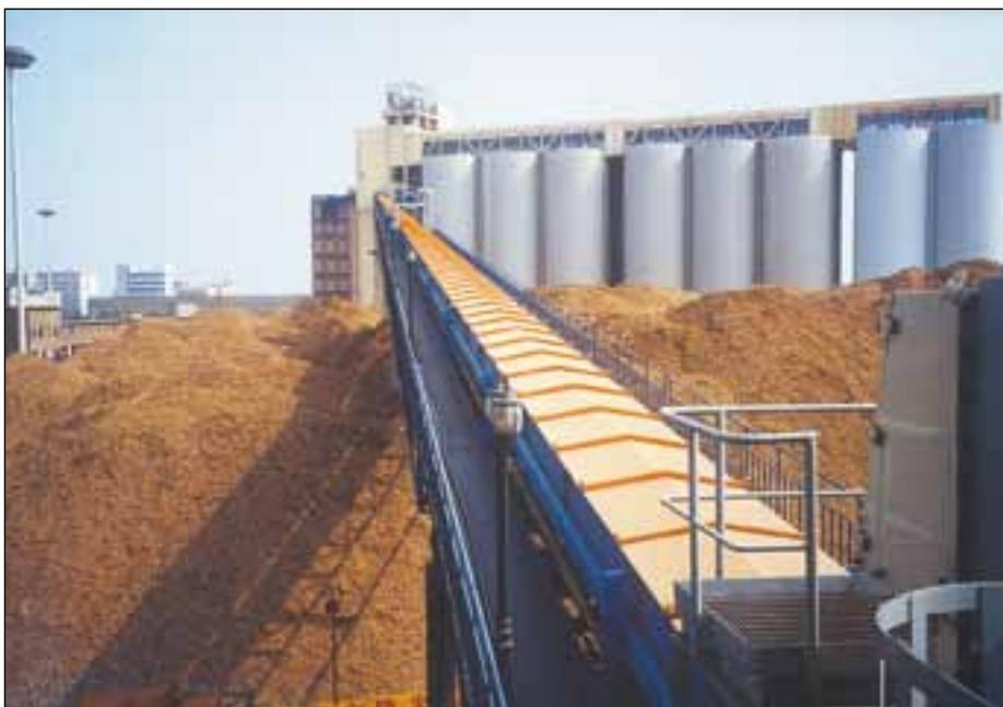
Air supported conveyor linking the wharf conveyor to the storage silo for processing.
