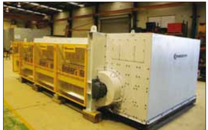
Picture shows the compactness of the LPF: the vertical distance between belt surface and underside of foot plates is only 1.2m.
