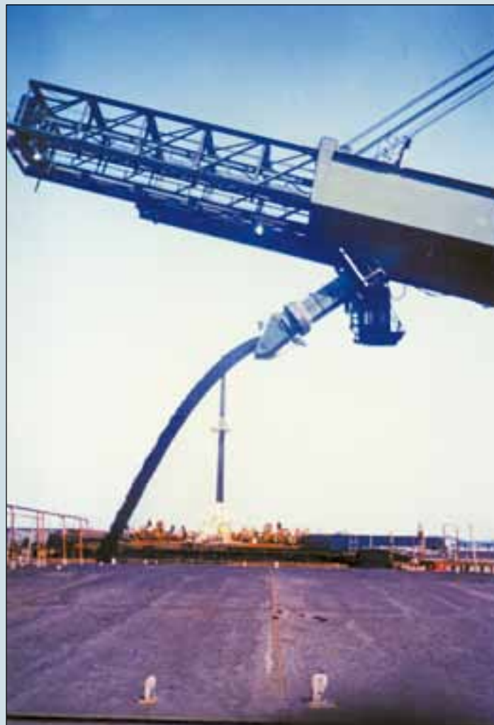
RG Tanna Coal Terminal Shiploader – first application of CFMSTS®.
