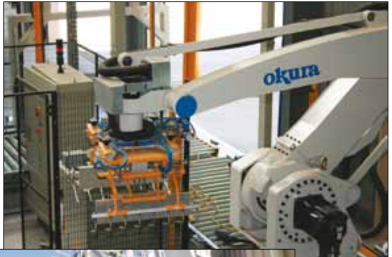
The Okura A1600 II robot palletizer is capable of accurately placing 1600 bags per hour.
