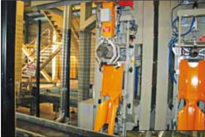
Bag placers: the fully automated Weitek four head valve bag filling station is equipped with automatic bag placement and is capable of 24 TPH.
