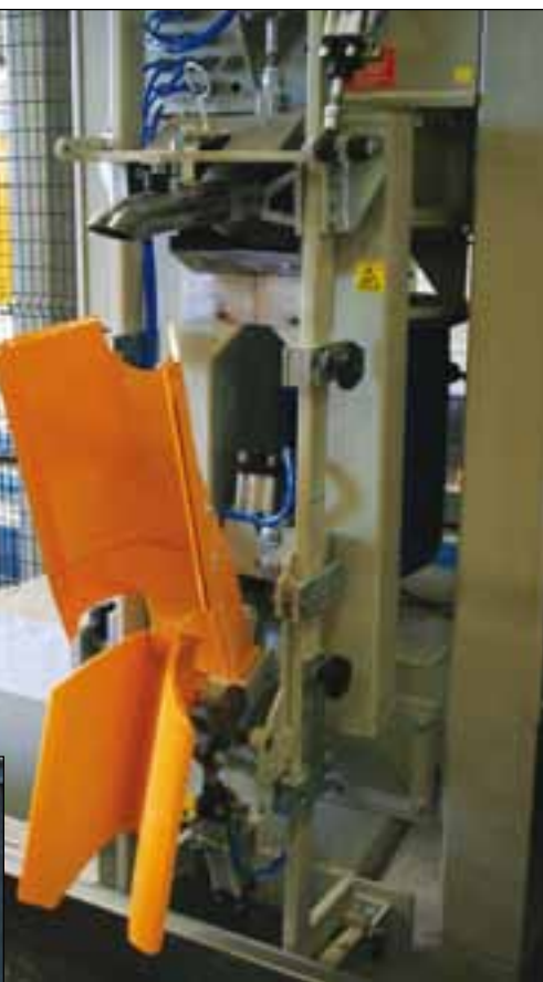
Weitek bagger: after being filled the bags are lowered to transfer conveyors for cleaning and check weighing prior to palletizing and stretch wrapping.
