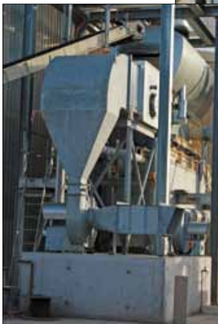
Sand dryer: the gas fired energy efficient Ventilex unit combines drying and cooling in the fluid bed drier process at 20 TPH of sand to a preset moisture content.
