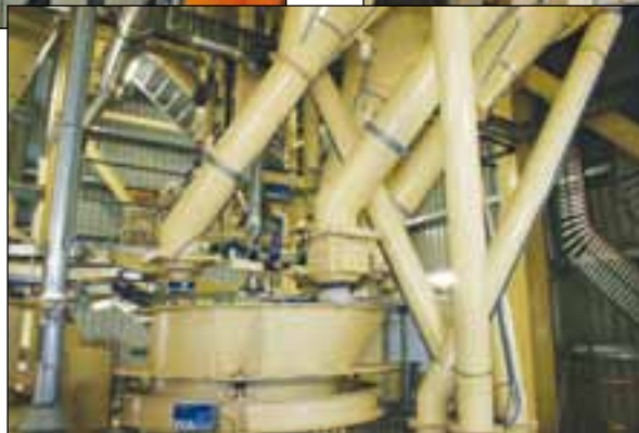
Weigh hoppers: raw materials are loaded into the weigh hoppers with high accuracy via the patented double flap dosing valves prior to being batched to the mixer.
