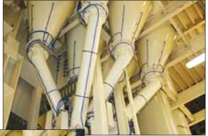
The fluidization system ensures efficient fluidization by introducing a small amount of air through the patented elements to ensure even, efficient material flow.
