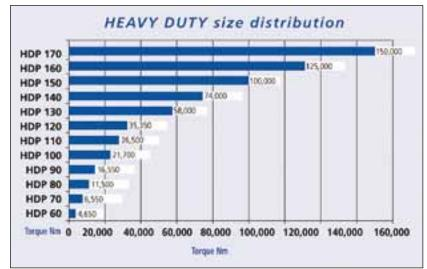
HDP size chart showing the torque output in Nm of the different sizes of HDP helical drives.
