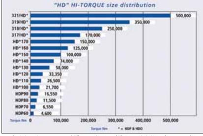
Graph shows the torque outputs of different combinations of HD drives, with the highest four outputs relating to combinations of HD helicals and Trasmital planetaries.
